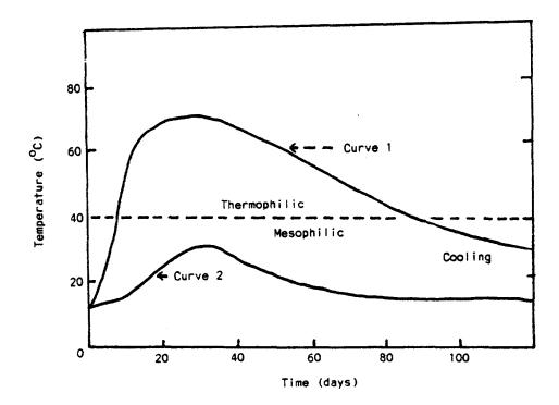
Figure 2. A typical time/temperature relationship for composting sewage sludge by the aerated pile method. Curve I depicts a situation where conditions of moisture, temperature, and aeration are at optimum levels for rapid transition from the mesophilic into the thermophilic stage. Curve 2 represents a condition where certain parameters are deficient or outside their optimum range, resulting in adverse effects on the growth and activity of the indigenous organisms.
