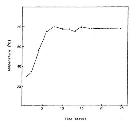
Figure 1. Typical time/temperature relationship using mode values of readings taken at 14 monitoring points within each of 12 static piles.
